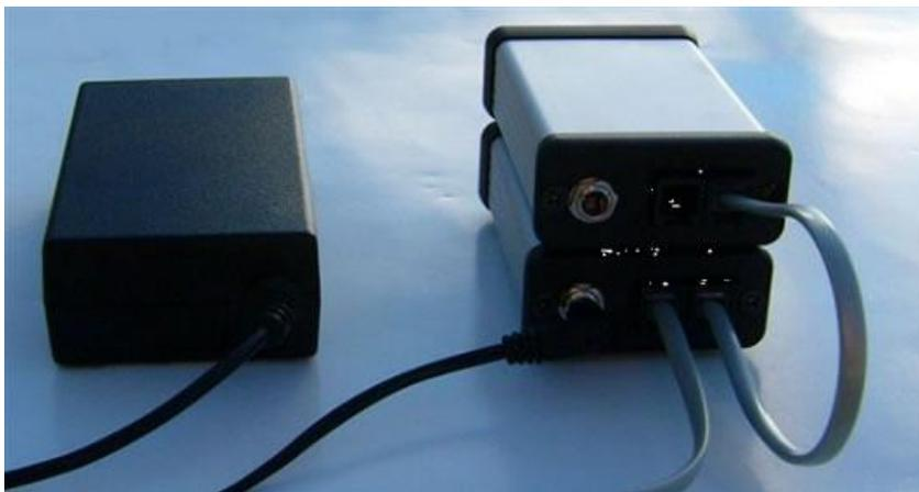
**Figure 2:** Back view and connection of two MC-101-01, only one power supply is necessary.
