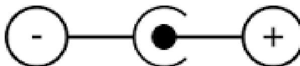
**Figure 3:** Connection Polarity.
