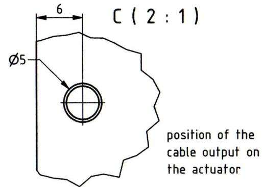
position of the cable output on the actuator
