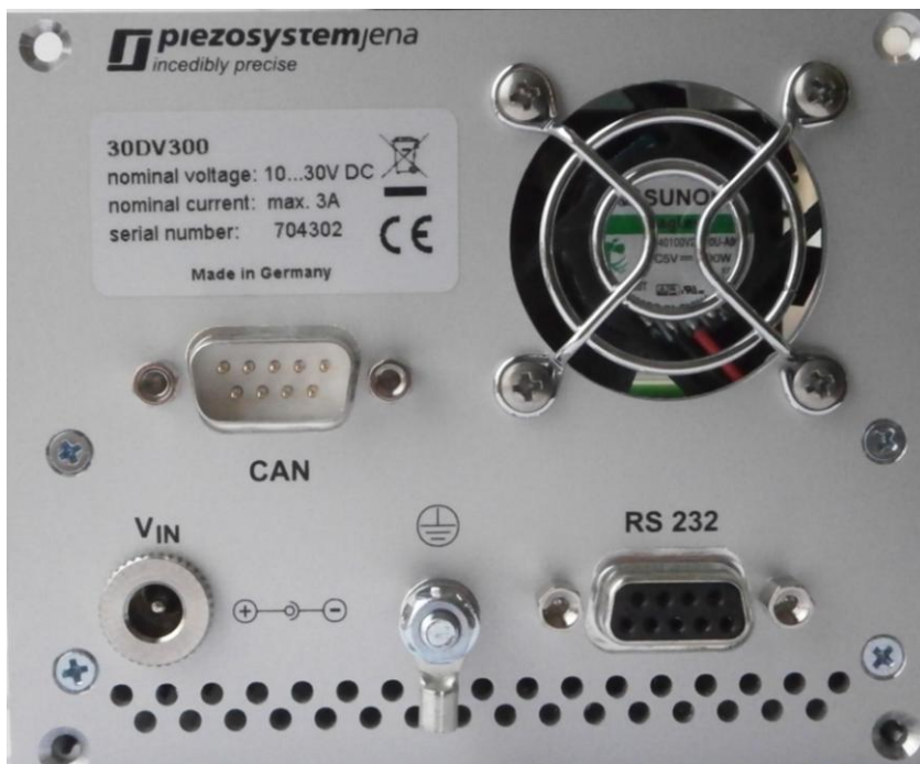
pic: view of the back panel with interfaces: Power (Vin), CAN and RS232
